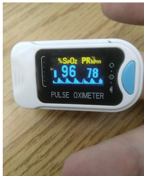
Figure 2: A pulse oximeter using photoplethysmography for heart rate and SpO2 measurement
